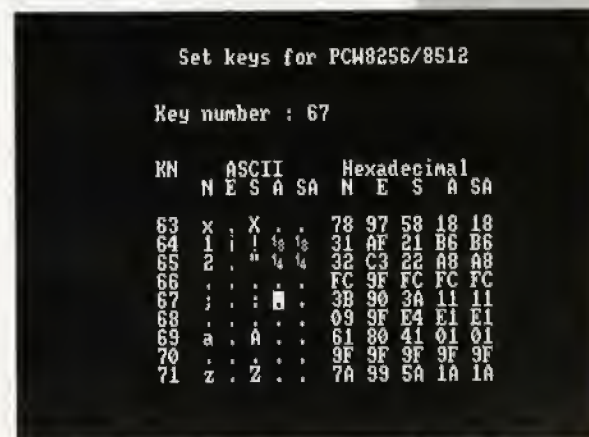
With the setkeys menu you will be able to change the characters stored under any of the keys on the keyboard
